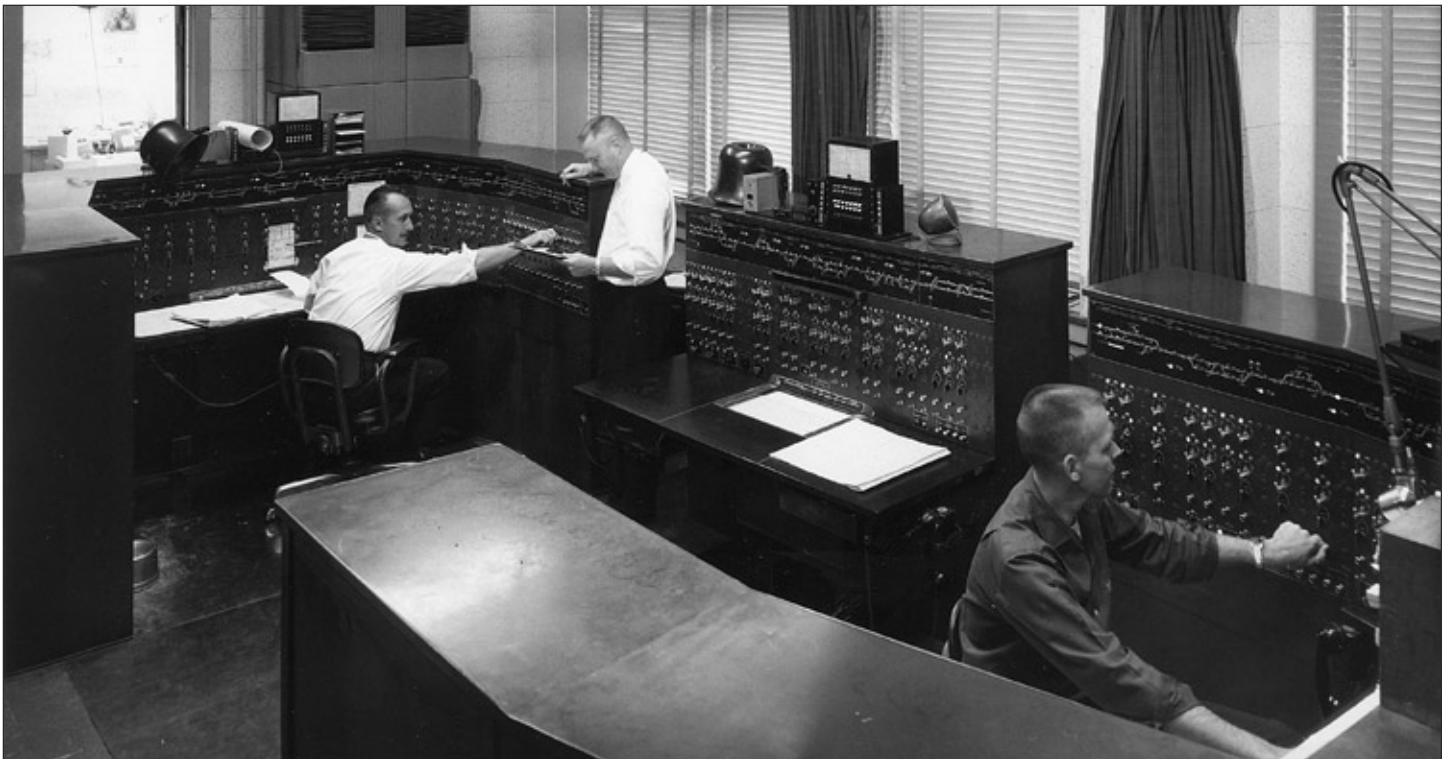
Here is the dispatcher's office in the Santa Fe building in Amarillo about 1962. The Third District machine is in the background. To its right is the Second District "pup" which controlled from Pampa to Mendota and the large Second District machine controlling from Waynoka to Canadian at far right. The First District machine (Wellington to Waynoka) is located in another room.
